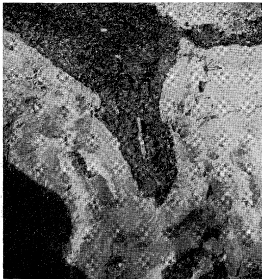
Pl. 1. A wedge-shaped intrusion of the dark-grey glacial silt, containing a sea molusca and foraminifera, into the underlying fine-grain sands (convection subsidence of the second phase of instability)
