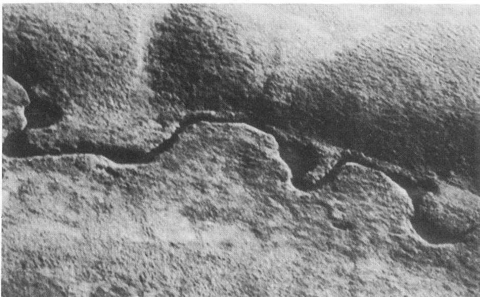
Figure 2. Beaded stream . Air view from an altitude of about 300 m in continuous permafrost zone near Tuktoyaktuk, N.W.T. (From Brown, 1970b. University of Toronto Press 1970)
